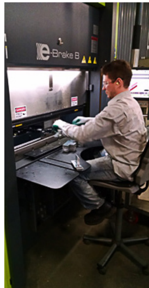
An Operator at Rough Brothers forming two brackets at once on the Safan Electric Brake without using the foot pedal.
