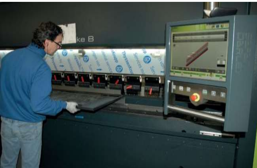
Working on one of the new SafanDarley E.Brake 100 – 3100 electric press brakes acquired by Larinox and installed at their sheet metal processing site.
